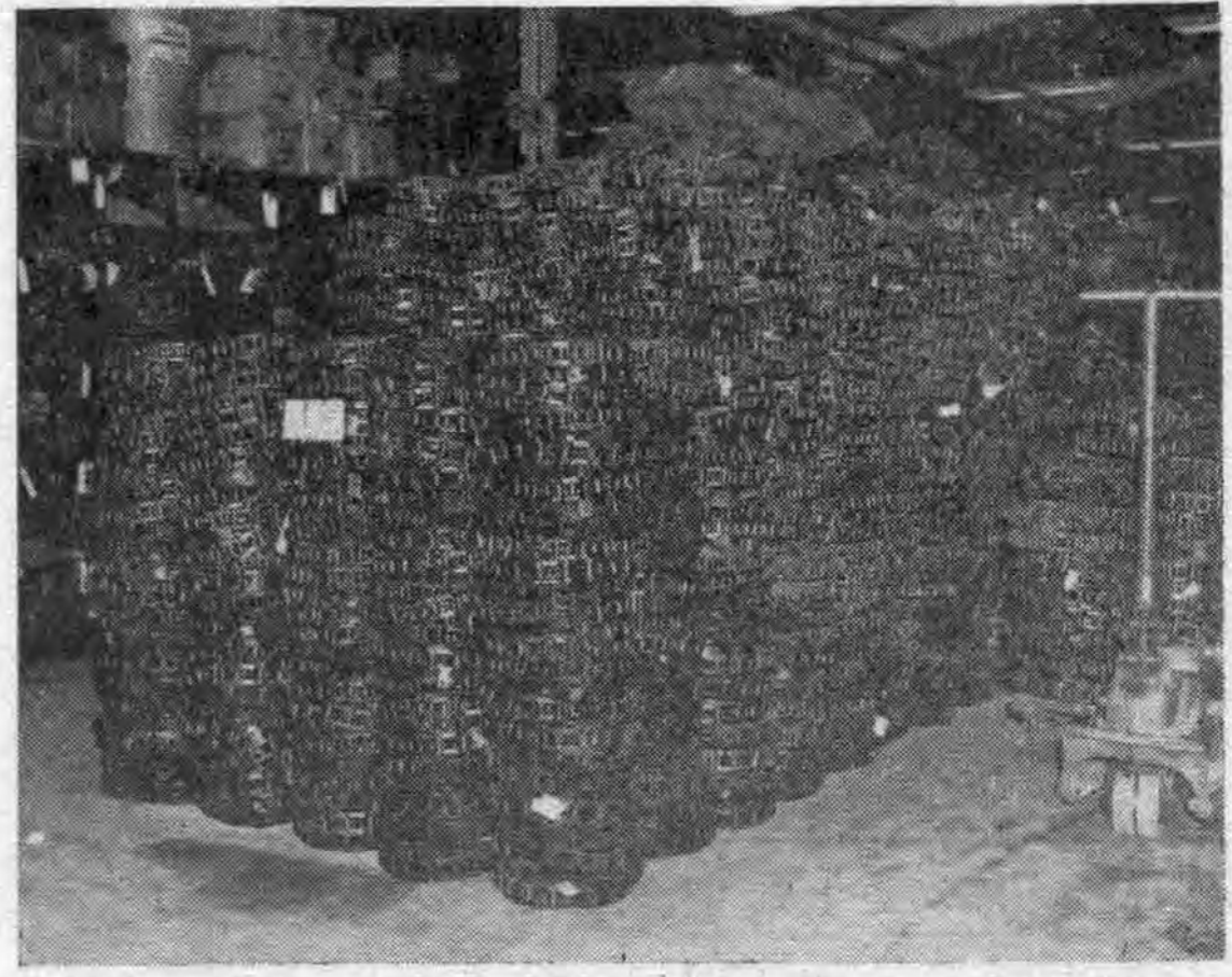
RIGHT —Photo of chain correctly stored. Note how the bundles of chain are piled evenly and perfectly vertical so as to avoid shifting or a leaning position. It may be seen that the stacks on the outside are not so high. This lessens the possibility of them falling, should the stack be jarred or bumped. The neat and orderly stacking presents a good housekeeping gesture.
